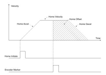
Figure 34: \Home to Marker Profile (Specified Offset)
